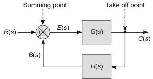
**Fig. :** Block diagram of closed-loop system
